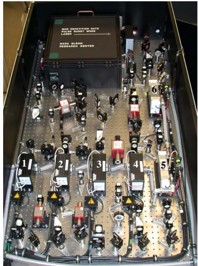
Figure 2: Photograph showing layout of pulse burst laser components on optical breadboard (enclosure cover removed).
