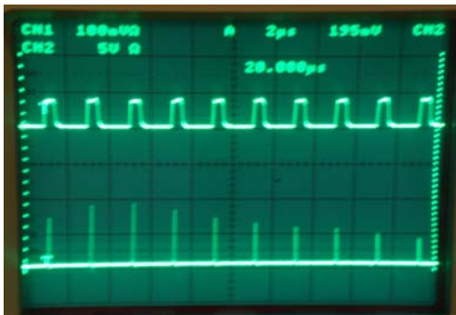
Figure 3: Oscilloscope trace of typical 10 pulse train illustrating envelope modulation. The top trace is the electric signal sent to the pulse slicer and the bottom trace is the actual laser output energy.
